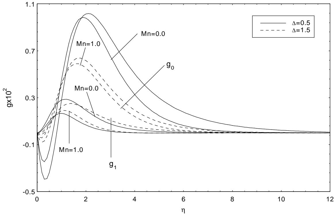
Fig.9. Microrotation profiles for adiabatic surface with concentrated heat source along the horizontal leading edge, a wall plume.
