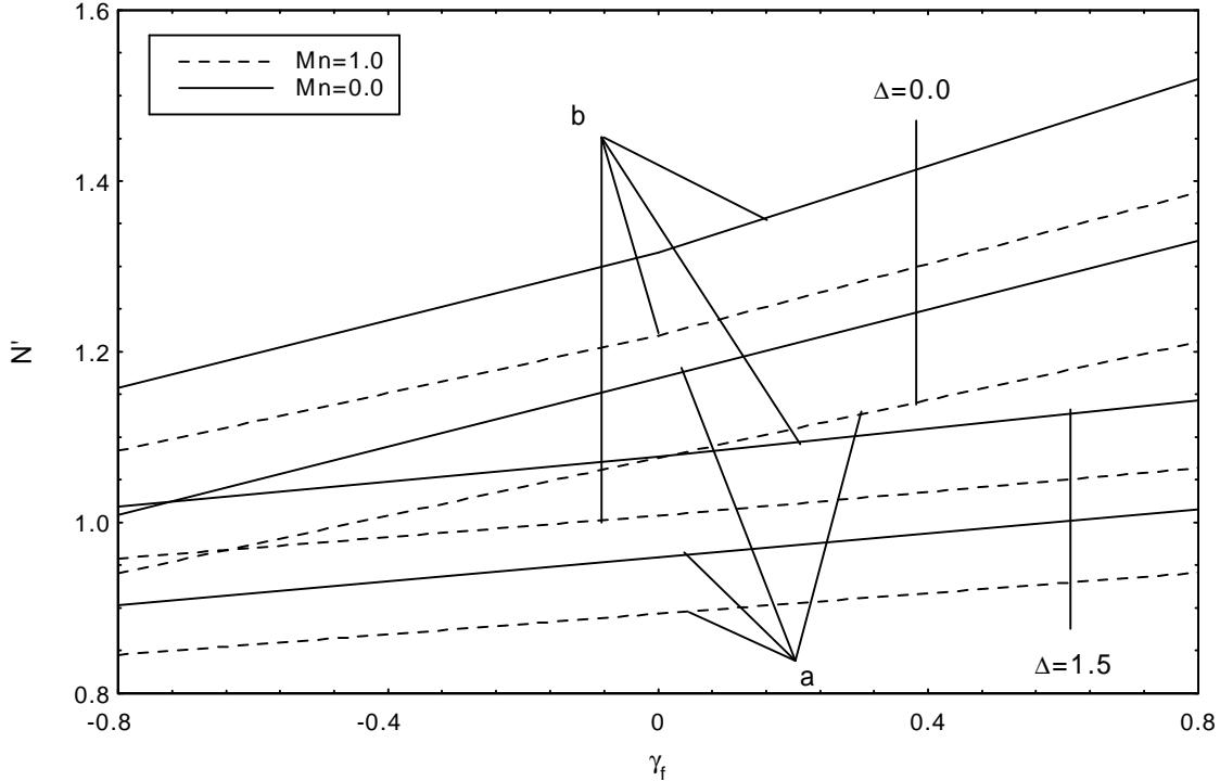
The effect of  $\gamma_f$ ,  $R$  and  $\Delta$  on heat transfer, for isothermal condition (a) and uniform heat flux (b). Fig.13.
