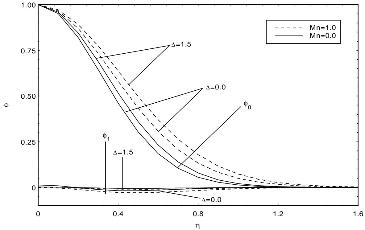
Fig.11. Temperature profiles for unbounded plane plume, rising from a horizontal thermal source at  $x=0$ .
