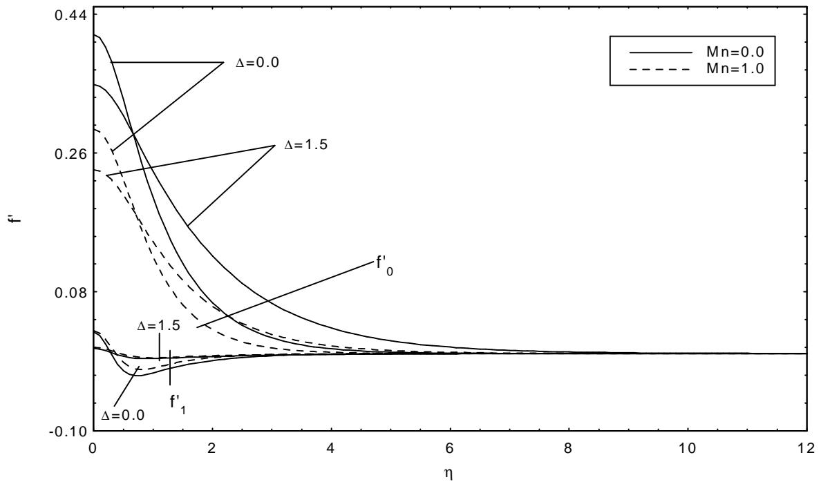
Fig.10. Velocity profiles for unbounded plane plume, rising from a horizontal thermal source at  $x=0$ .
