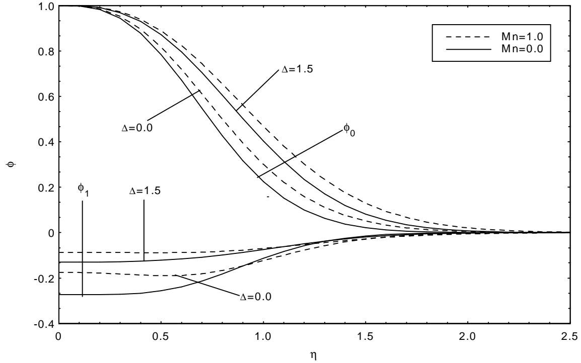
Fig.8. Temperature profiles for adiabatic surface with concentrated heat source along the horizontal leading edge, a wall plume.
