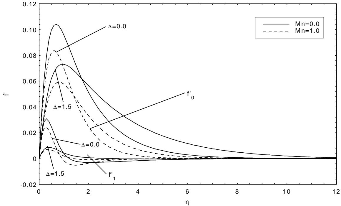
Fig.4. Velocity profiles for constant flux surface with horizontal leading edge.
