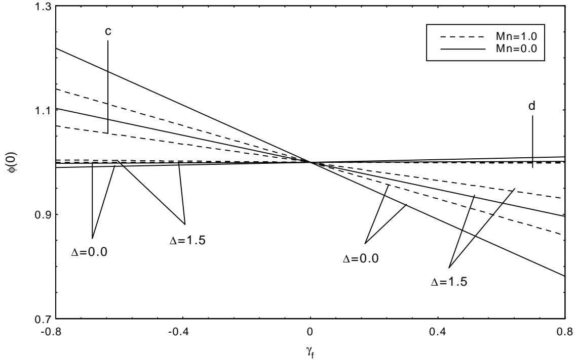
The effect of  $\Delta$  on transport,  $\phi(0, \gamma_f)$  for the adiabatic flows as a function of  $\gamma_f$  (c) plane plume, Fig.14.
