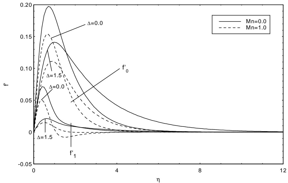
Velocity profiles for adiabatic surface with concentrated heat source along the horizontal leading edge, Fig.7.
