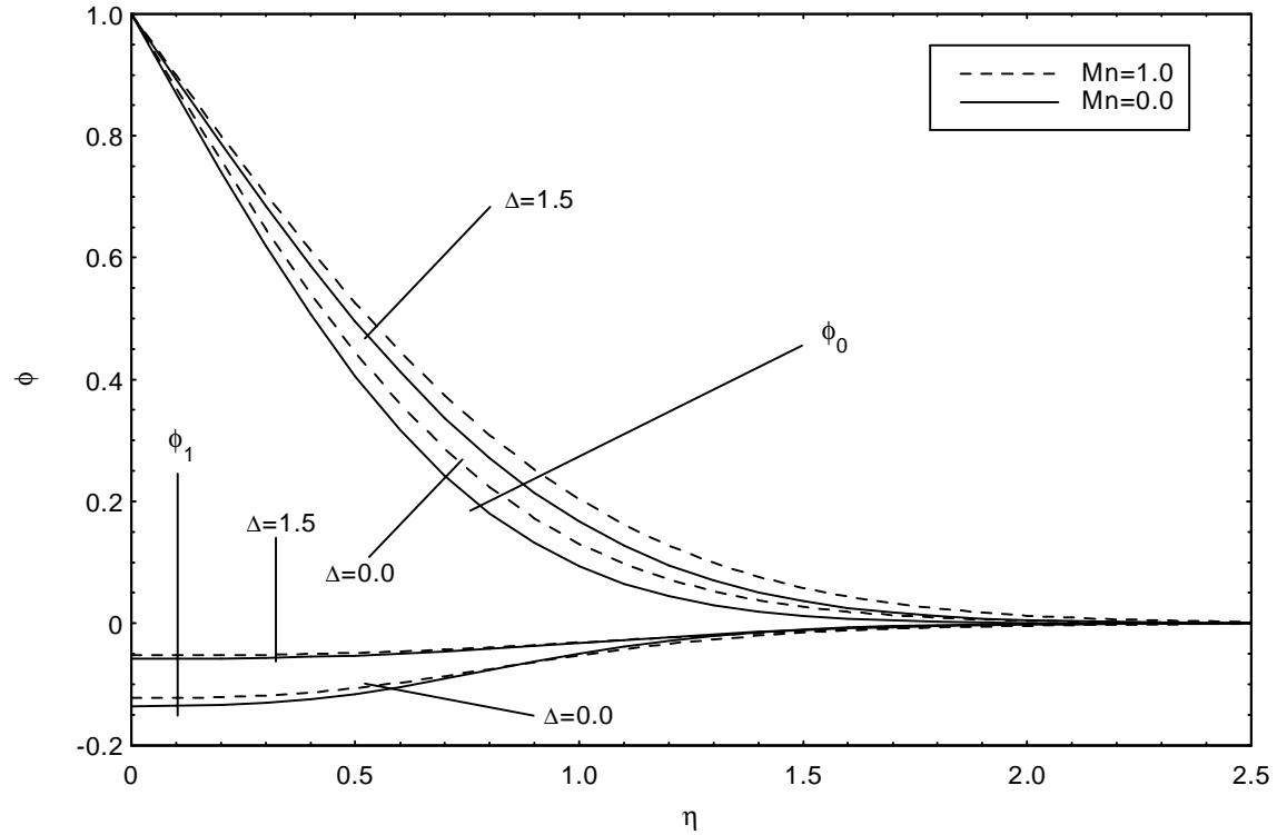
Fig.5. Temperature profiles for constant flux surface with horizontal leading edge.
