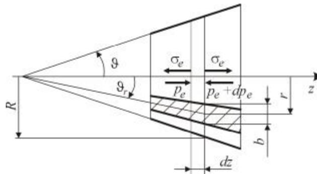
Fig.3. Schematic diagram of forces for the analysis of the pressure drop due to extensional flow.
