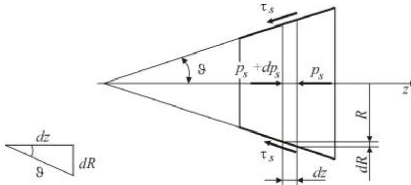
Fig.2. Schematic diagram of forces for the analysis of the pressure drop due to telescopic shear.
