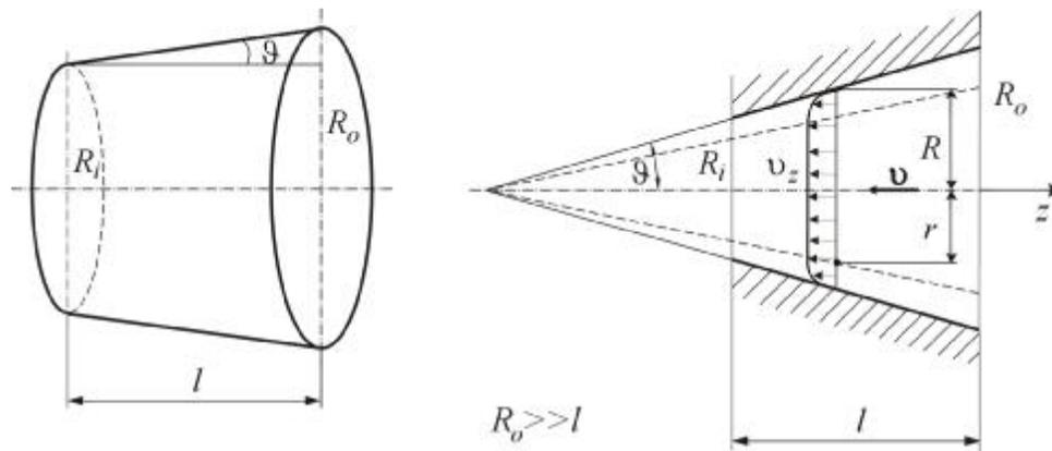
Fig.1. Schematic diagram of a conical flow.
