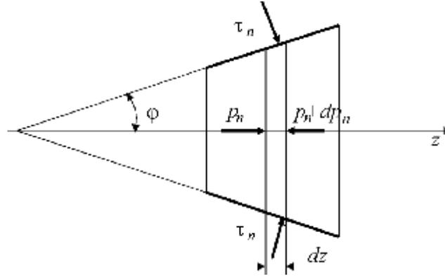
Fig.4. Schematic diagram of forces for the analysis of the pressure drop due to normal stresses.
