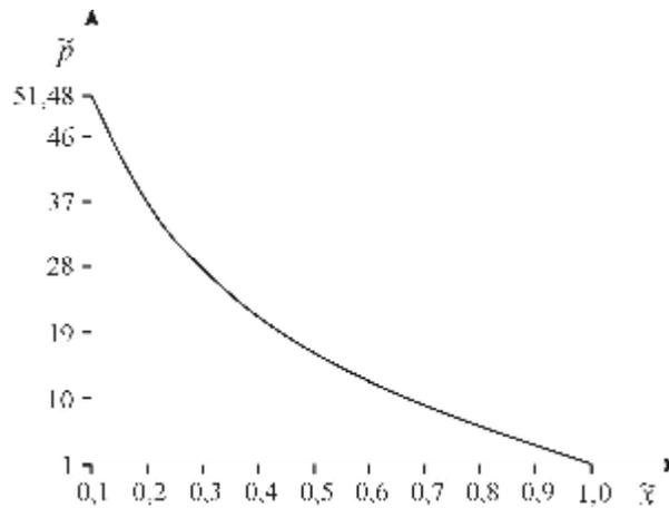
Fig.7. Dimensionless pressure distribution for a Bingham fluid and large  $K$ .
