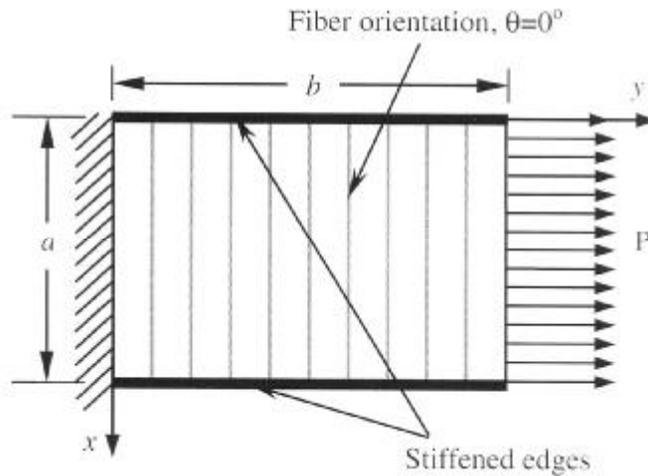
Fig.2. A flat composite bar with two opposing edges stiffened, under uniform axial loading.
