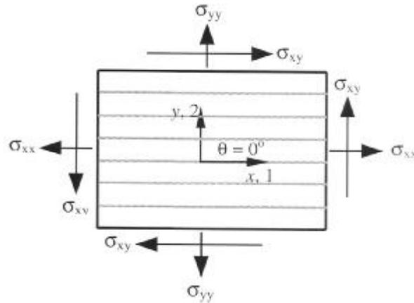
Fig.1. Stress components on a plane of an orthotropic composite material.
