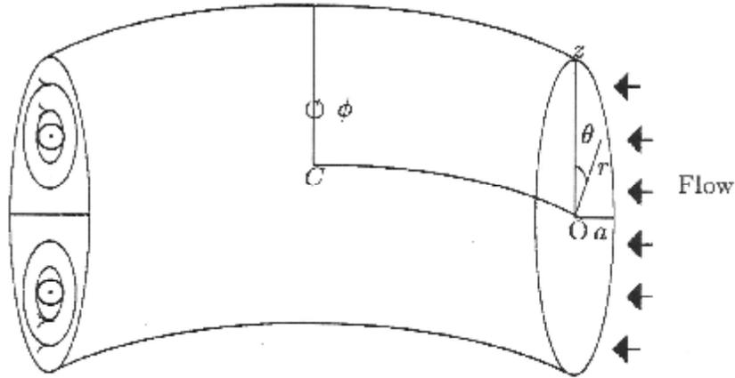
Fig.1. A schematic diagram of the flow in a curved pipe.
