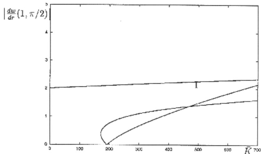
Fig.3. Approximate solution diagram (curve I) for  $\bar{K} > 0$  obtained by the Drazin-Tourigny (1996) method for  $d = 5$ . The other curves are spurious.
