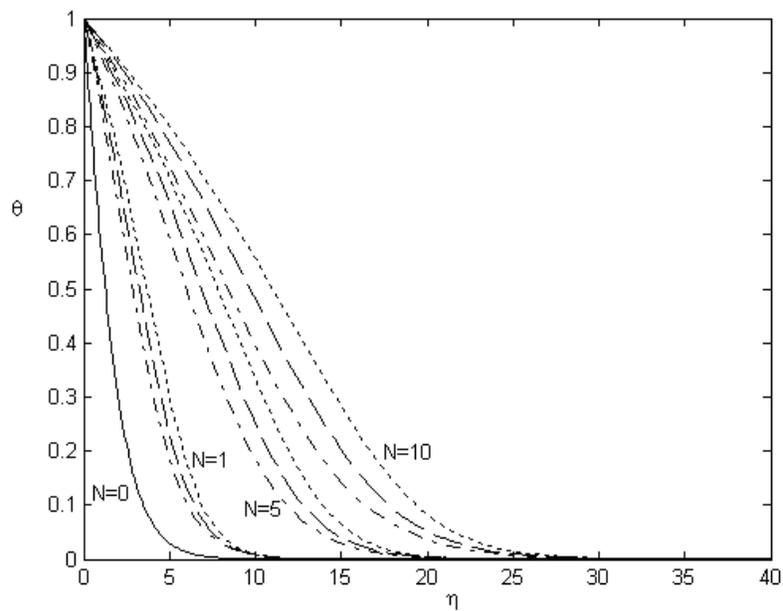
Fig.3. Dimensionless temperature profiles for  $n=1$ ,  $N=0, 1, 5, 10$  and  $\theta_w = 1.1(-\cdot-)$ ,  $1.5(---)$  and  $2(\dots)$ .
