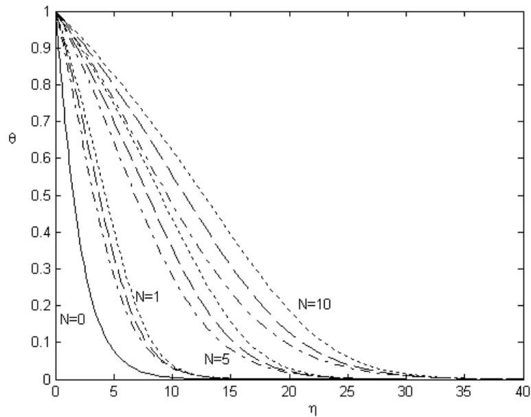
Fig.2. Dimensionless temperature profiles for  $n = 0.5$ ,  $N = 0, 1, 5, 10$  and  $\theta_w = 1.1(\text{---})$ ,  $1.5(\text{- - -})$  and  $2(\text{.....})$ .
