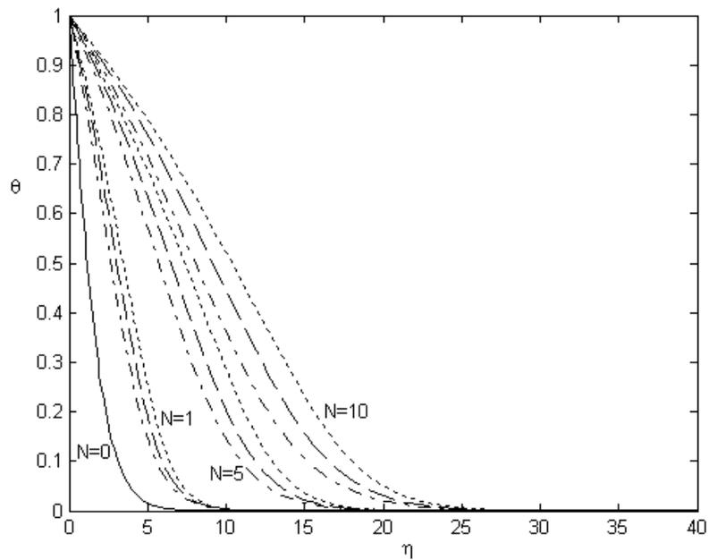
Fig.4. Dimensionless temperature profiles for  $n=1.5$ ,  $N=0, 1, 5, 10$  and  $\theta_w = 1.1(-\cdot-)$ ,  $1.5(---)$  and  $2(\dots)$ .
