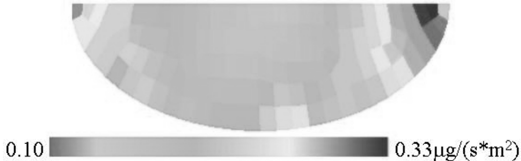
Fig.12. Total erosion wear rate of the wall material of the scattering element in \mu\text{g}/(\text{s} \times \text{m}^2) for the wear model III.
