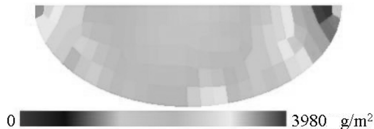
Fig.15. Erosion wear distribution in the wall of the scattering element obtained from numerical calculations after 7320 hours of service.
