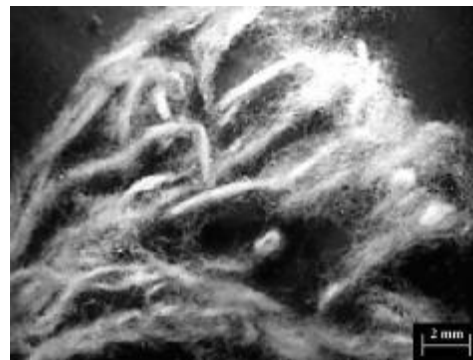
Fig.11. A group of pills (severe abrasive wear).
