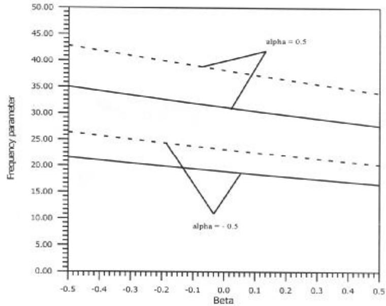
Fig1. (C-C conditions) Variation of first mode of frequency parameter with density parameter. (Soild curve – Orthotropic plate, Dashed curve – Monoclinic plate).
