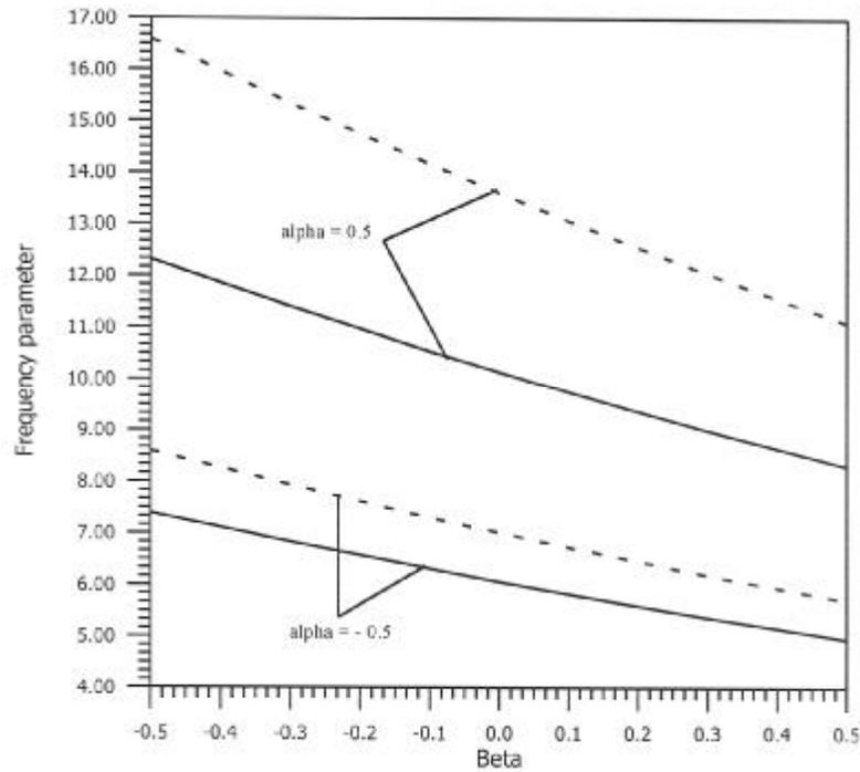
Fig.9. (*C-F* conditions) Variation of first mode of frequency parameter with density parameter. (Solid curve – Orthotropic plate, Dashed curve – Monoclinic plate).
