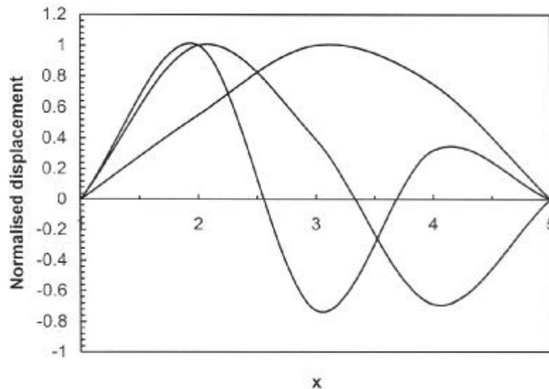
Fig.14. ( $C-S$  condition) Normalized displacements of monoclinic plate for the first three modes of vibrations.
