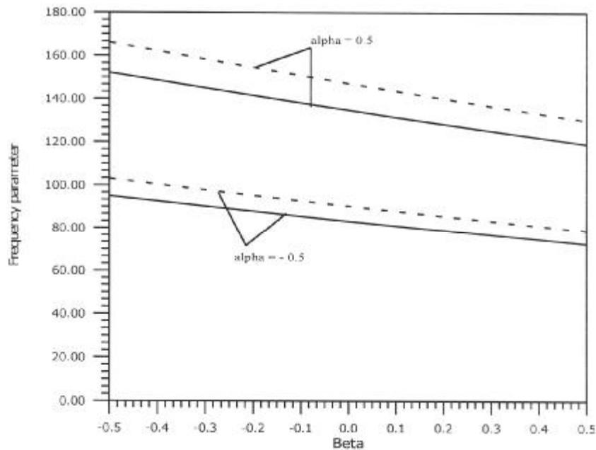
Fig.7. (C-S conditions) Variation of third mode of frequency parameter with density parameter. (Solid curve – Orthotropic plate, Dashed curve – Monoclinic plate).
