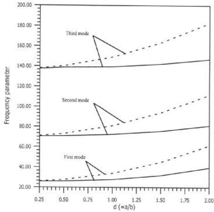
Fig.4. (C-C conditions) Variation of frequency parameters with aspect ratio. (Solid curve – orthotropic plate, Dashed curve – Monoclinic plate,  $\alpha = \beta = 0.5$ ).
