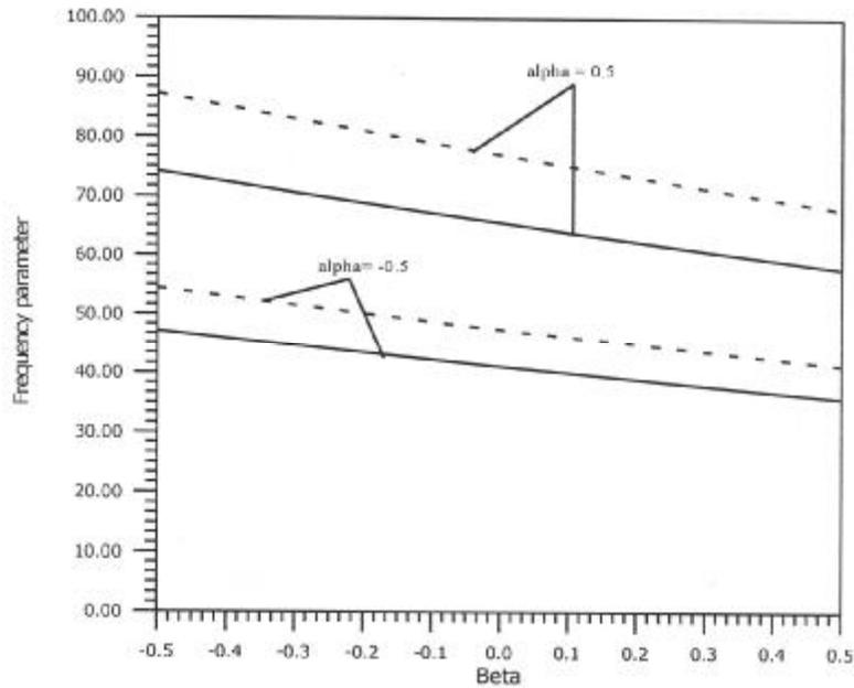
Fig.6. (C-S conditions) Variation of second mode of frequency parameter with density parameter. (Solid curve – Orthotropic plate, Dashed curve – Monoclinic plate).
