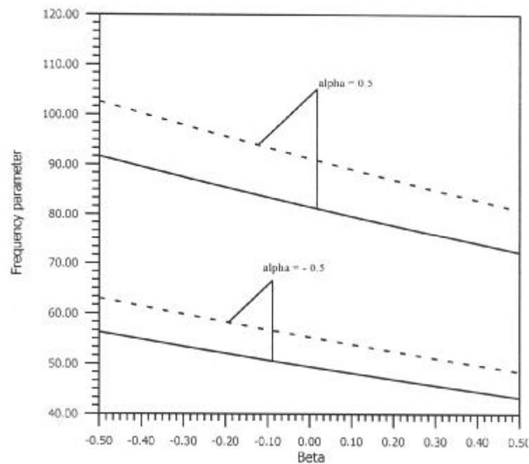
Fig.2. (C-C conditions) Variation of second mode of frequency parameter with density parameter. (Soild curve – Orthotropic plate, Dashed curve – Monoclinic plate).
