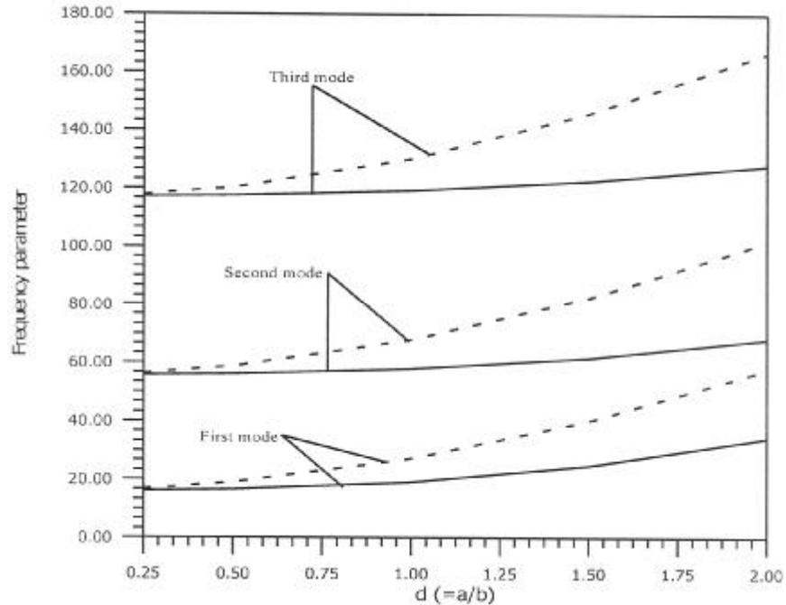
Fig.8. (C-S conditions) Variation of frequency parameters with aspect ratio. (Solid curve – orthotropic plate, Dashed curve – Monoclinic plate,  $\alpha = \beta = 0.5$ ).
