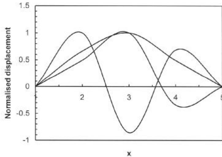
Fig.13. ( $C-C$  condition) Normalized displacements of monoclinic plate for the first three modes of vibrations.
