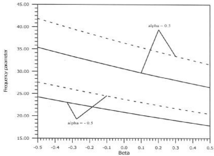
Fig.10. (*C-F* conditions) Variation of second mode of frequency parameter with density parameter. (Solid curve – Orthotropic plate, Dashed curve – Monoclinic plate).
