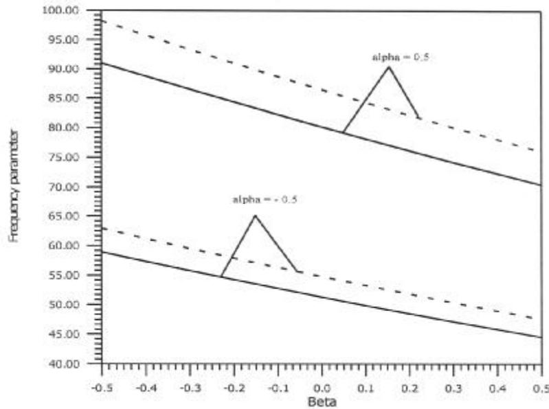
Fig.11. (C-F Conditions) Variation of third mode of frequency parameter with density parameter. (Solid curve – Orthotropic plate, Dashed curve – Monoclinic plate).
