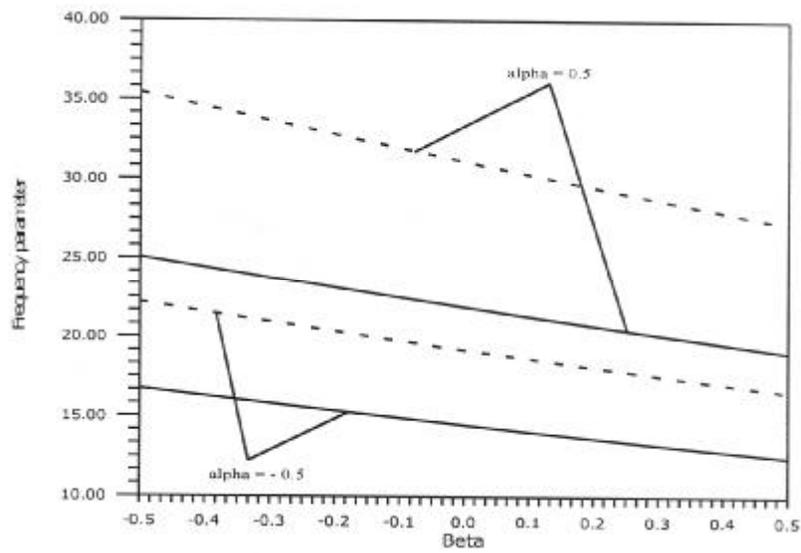
Fig.5. (C-S condition) Variation of first mode of frequency parameter with density parameter. (Solid curve – Orthotropic plate, Dashed curve – Monoclinic plate).
