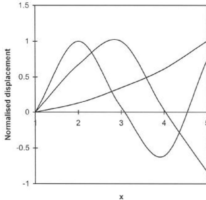
Fig.15. (*C-F* condition) Variation of normalized displacements with  $X$  in monoclinic plate for the first three modes of vibrations.
