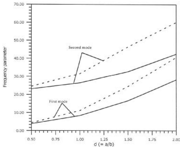
Fig.12. (C-F conditions) Variation of frequency parameters with aspect ratio. (Solid curve – orthotropic plate, Dashed curve – Monoclinic plate,  $\alpha = \beta = 0.5$ ).
