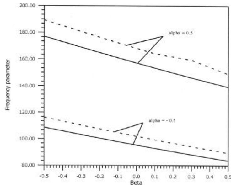
Fig.3. ( $C-C$  conditions) Variation of third mode of frequency parameter with density parameter. (Solid curve – Orthotropic plate, Dashed curve – Monoclinic plate).
